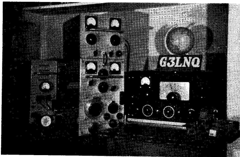
The station of G3LNO—ex-ZL2GQ, and now at 5 Hillfield Close, North Harrow, Middlesex—is entirely home-built, including the receiver, which is to a design originally published in "Short Wave Magazine." The G3LNO transmitter has been selected for discussion in the accompanying article, with some notes on the station generally.
